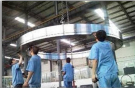
Bearing E8331-7P in assembling
